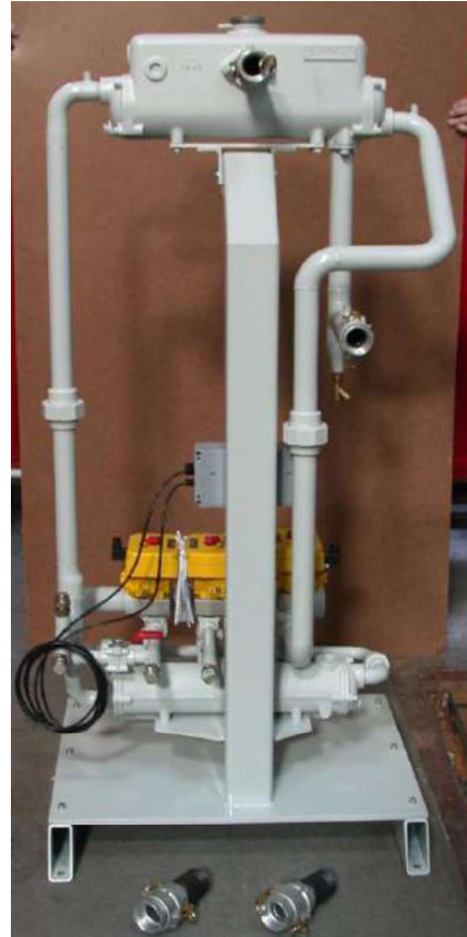
Cooling Post Module with Valve Manifold Assembly Located at base, Bowman Engine Header tank Heat Exchanger on top and Oil Heat exchanger at low level.
