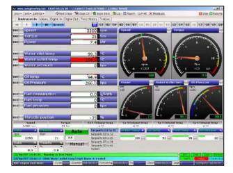
provide additional test stages or Transient Schedules can be called from within a test. A Transient Schedule is a schedule of pre-written setpoints in a prescribed format within an Excel spreadsheet.
